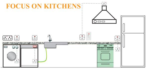
555.2.1 In domestic and similar installations, an isolating device for a cooking appliance shall not be mounted either directly above or behind the appliance.
