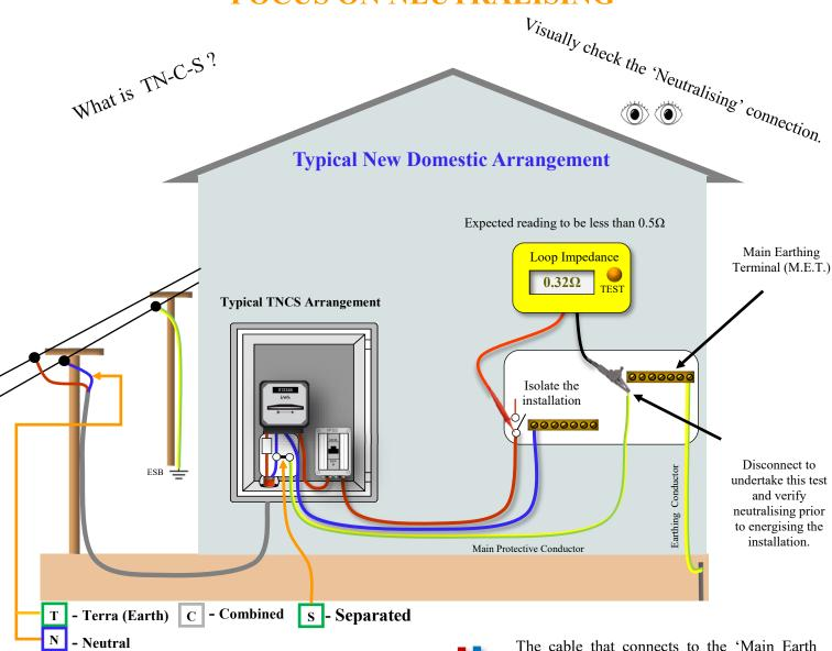
Almost the entire country uses the TNCS wiring system. (Terra Neutral Combined & Separate). With this system, on the ESB's side of the installation i.e. before the electricity meter the Neutral and Earth are combined into one conductor. On the Customer side i.e. after the electricity meter the Neutral and Earth are separated into two conductors.
