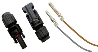
DC connectors (typically MC4) must be rated to IP21, class II, shrouded and must be labelled positive and negative.
